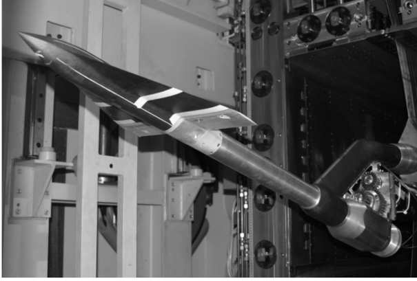
Fig. 3 Configuration of 65 deg swept delta-wing-fuselage model with remote-controlled trailing-edge flaps on the roll-rig device in the DNW-TWG Göttingen.
